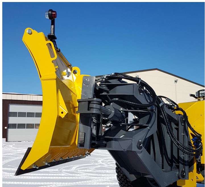
Front blade – up/down, turning and with a leaning system, a safety box for blade edges and a support arm
