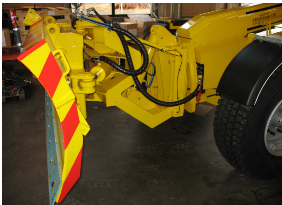
Front blade – up/down, turning and with a leaning system, a safety box for blade edges and a support arm
