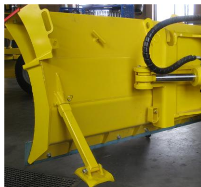
Front blade – up/down, turning and with a leaning system, a safety box for blade edges and a support arm
