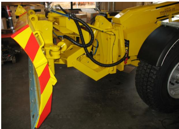
Front blade – up/down, turning and with a leaning system, a safety box for blade edges and a support arm
