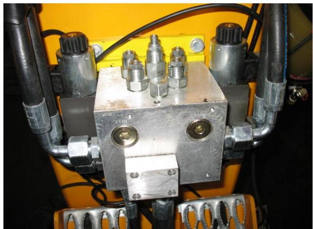
*Display/control unit (up on the right), one of the sensors of the blade tilting automatism (down on the left) and the valve kit required on RG motor graders (not required on FG motor graders)*
